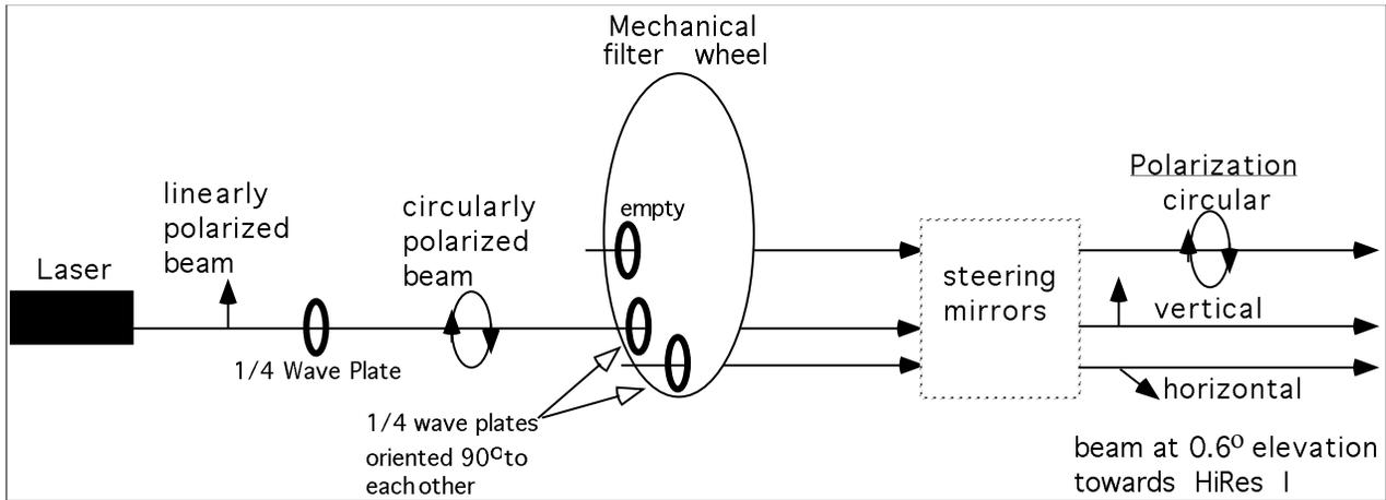
**Figure 2:** Schematic representation of polarizations available in HR2SLS. The steering mirrors consist of three dielectric mirrors that are positioned at 45° with respect to the incident laser beam.
