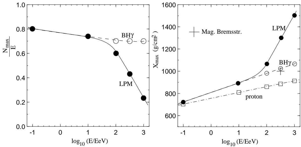
Figure 3: Effect of LPM and Magnetic Bremsstrahlung on Xmax and Nmax
