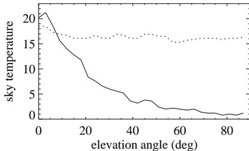
Figure 4: Sky temperature as a function of elevation angle for a clear sky (solid line) and a cloudy sky (dotted line).
