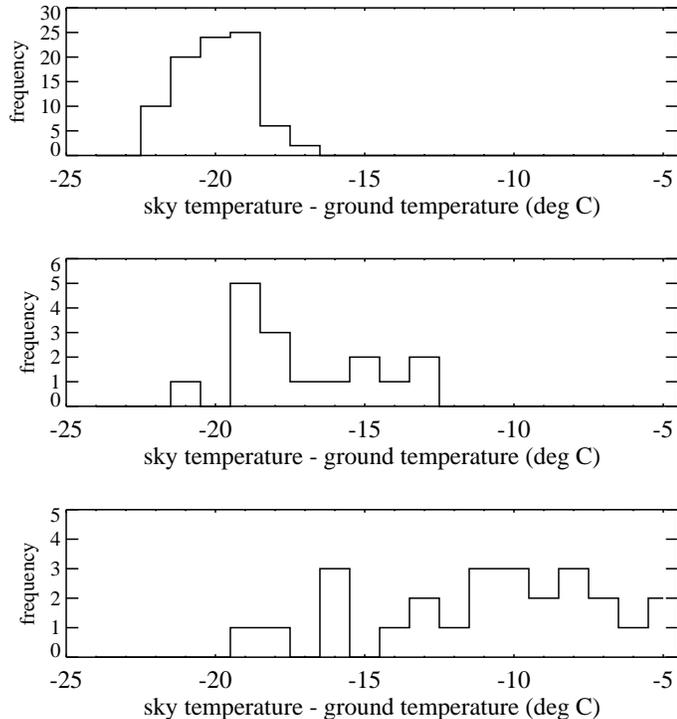
Figure 2: Difference between the sky and ground temperatures for March/April 1999 runs at Dugway. Operators classified the conditions as clear (top plot), thin cloud (middle plot) and cloudy (bottom plot).
