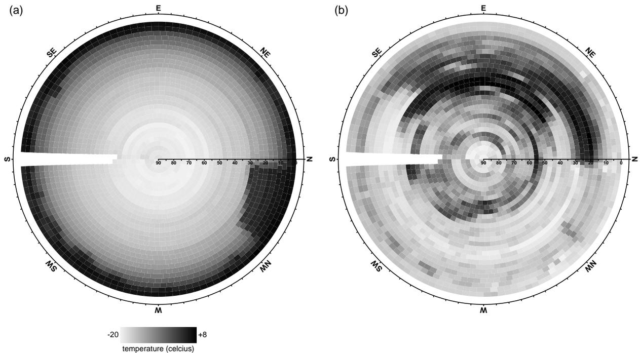
Figure 3: Sky images from scanning cloud monitor. (a) Clear sky with shading indicating sky temperature from -20 degrees C (white) to +8 degrees C (black). (b) Partly cloudy sky with clear sky zenith variation subtracted.
