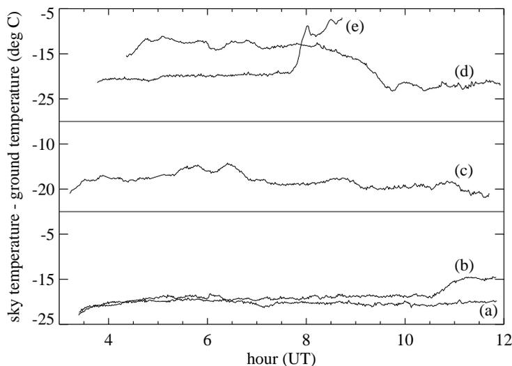
Figure 1: Examples of wide angle cloud monitor signals from Dugway in March/April 1999. Each line represents the difference between the measured sky temperature and the ground temperature. Large negative values represent clear skies. Details in Section 3.
