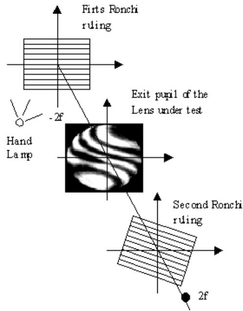
Figure 2a.- Testing a lens with Ronchi rulings of same frequency
