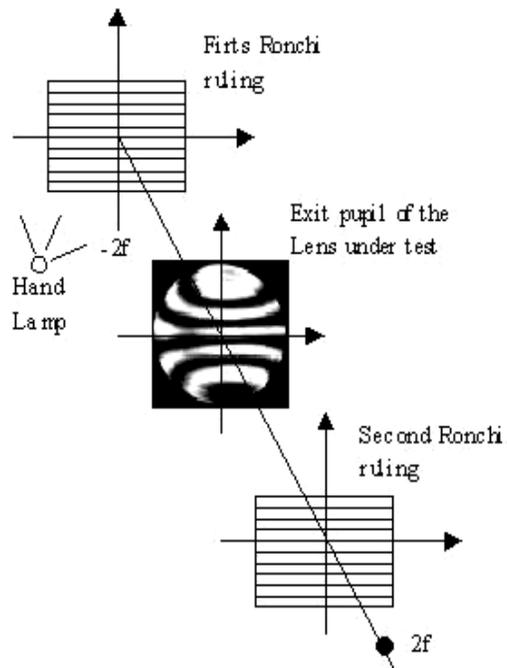
Figure 2b.- Testing a lens with Ronchi rulings of different frequencies.
