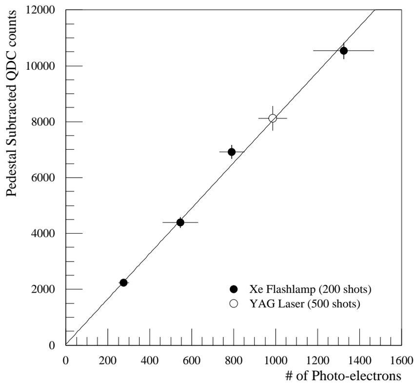
Gain fit for a single PMT
