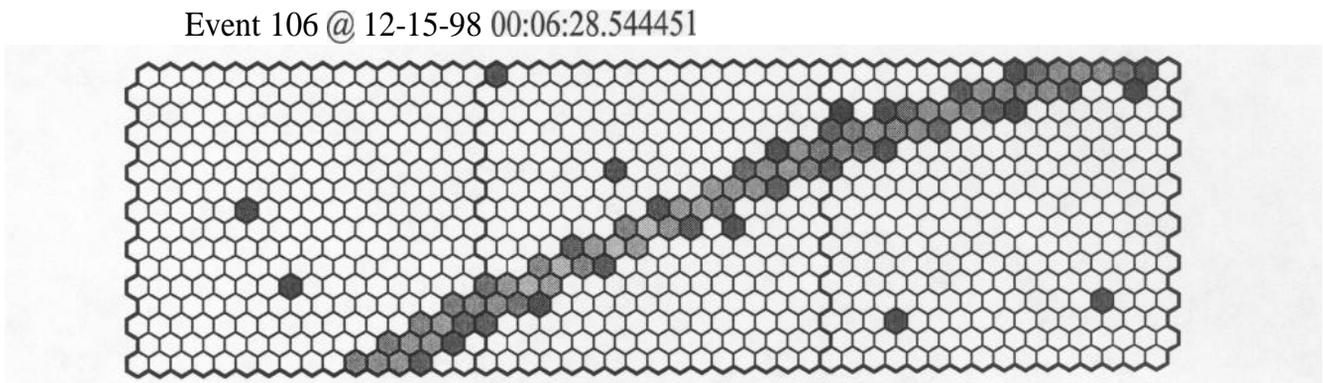
Figure 2: An event display for a laser shot seen in three mirrors.
