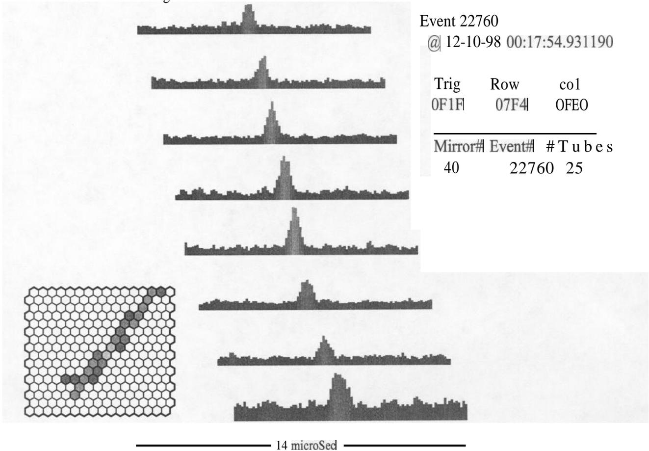
Figure 1: HiRes event display of a cosmic ray shower with FADC profiles for eight viewing channels.
