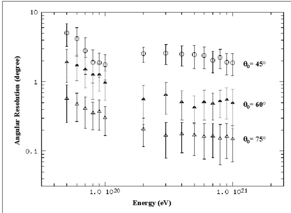
**Figure 3:** Results of the off-line event geometrical reconstruction. Angular resolution versus energy for events simulated at azimuth angle  $\phi_0=33^\circ$ , and zenith angle  $\theta_0=45^\circ$ ,  $60^\circ$ , and  $75^\circ$ , respectively.
