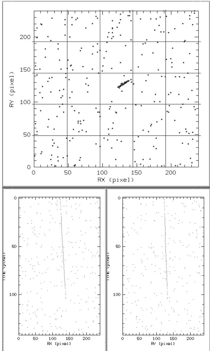
**Figure 1:** Visualization of a fluorescence signal. At the top: image of the event on the X-Y detector plane. At the bottom: the signal as viewed along the two projection planes (Time-X and Time-Y).
