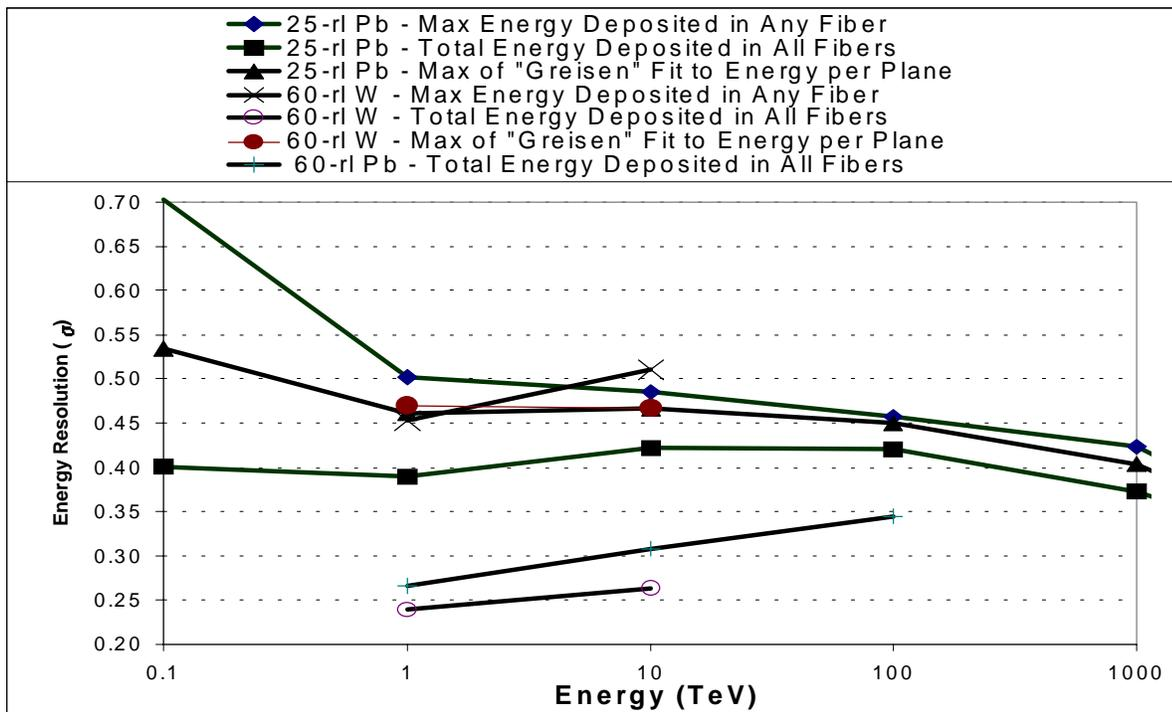
Figure 5. The calculated energy resolution for 25-rl lead and 60-rl lead and tungsten calorimeters, using three different methods for estimating energy.
