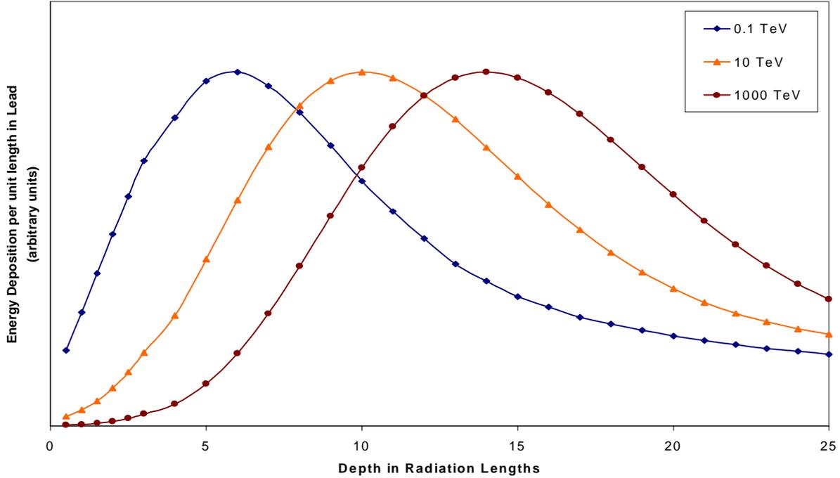
Figure 4. Average shower profiles for proton energies 0.1, 10, and 1000 TeV, with cascade maxima normalized. Deposited energy in calorimeter lead layers.
