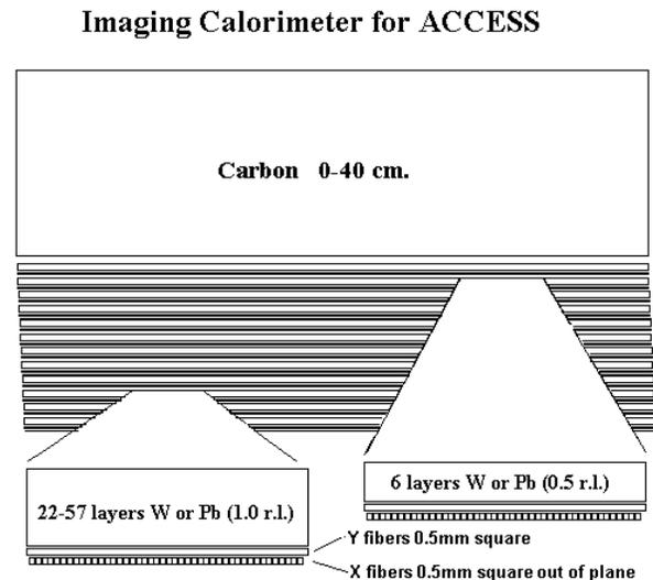
Figure 1. Imaging Calorimeter for ACCESS
