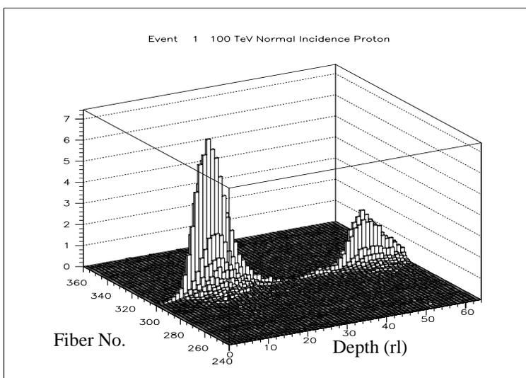
Figure 2. A cascade from a 100 TeV proton in a 60-rl calorimeter; energy per fiber in GeV
