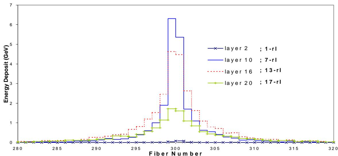
Figure 3. Energy deposition per fiber in GeV at various depths for a 100 TeV proton
