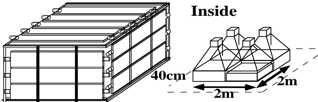
**Figure 2:** A schematic view of the solar neutron detector at Chacaltaya.
