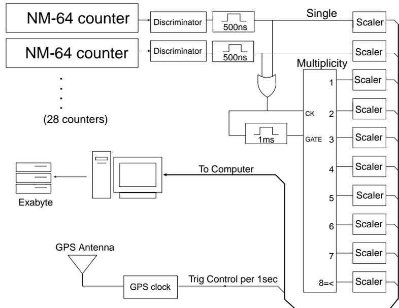
Figure 1: Block diagram of counter system for data acquisition.
