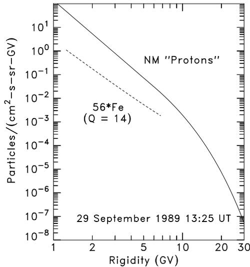
Figure 4: Fe and proton intensities as functions of rigidity. Fe rigidities are evaluated assuming ionic charge  $Q=14$ . The Fe intensity is also multiplied by a factor of 56, as discussed in the text. The solid proton curve is the Lovell et al. spectrum at 13:25 UT.
