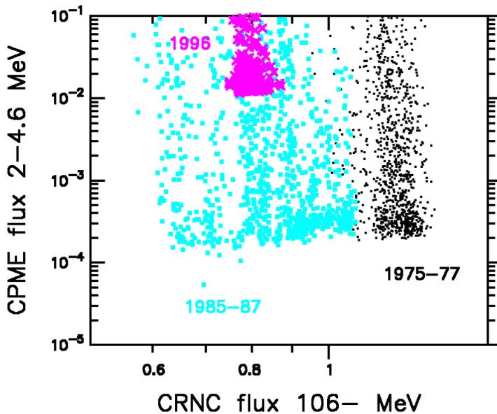
**Figure 2:** Scatter plot of daily flux ( $p/cm^2 s sr MeV$ ) averages of CPME 2-4.6 MeV protons vs. CRNC  $>106$  MeV protons in the last three solar minima (x -1996 data).
