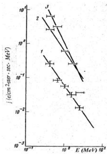
Fig. 2. Differential energy spectra of electrons: "background" spectrum (1); spectrum at the rise front (2); spectrum during the rise maximum (3).
