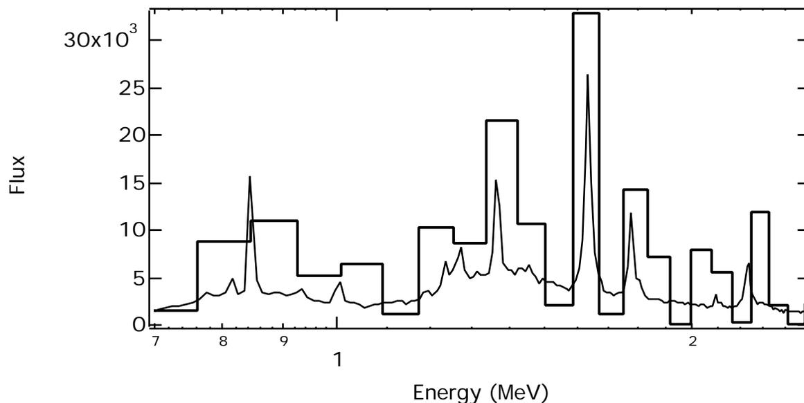
**Figure 2: The deconvolved photon spectrum with the theoretical spectrum superimposed over it.**
