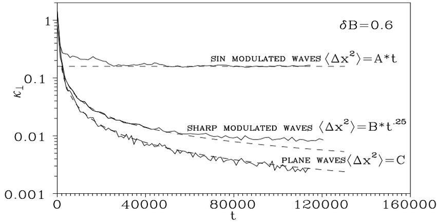
Figure 1: Examples of simulated  $\kappa_{\perp}$  versus the integration time  $t$ . The power-law fits of the cross-field particle dispersion  $\langle \Delta x^2 \rangle$  are presented for the model A and for the initial part of the curve for the model B2 ( $A$ ,  $B$  and  $C$  – constants). A constant fit is provided for the model B1.
