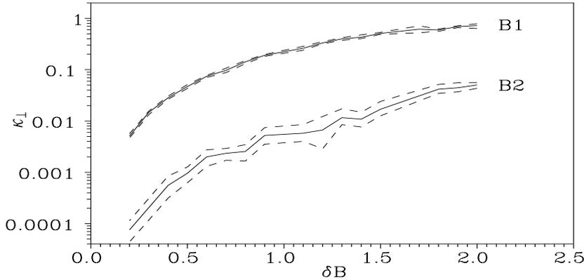
Figure 2: The simulated values of  $\kappa_{\perp}$  versus  $\delta B$  for the wave models B1 and B2. Solid lines join the results obtained using our fitting procedure. The adjacent dashed lines provide information about errors as they join the maximum (or respectively minimum) values of the quantity measured within the range used for fitting.
