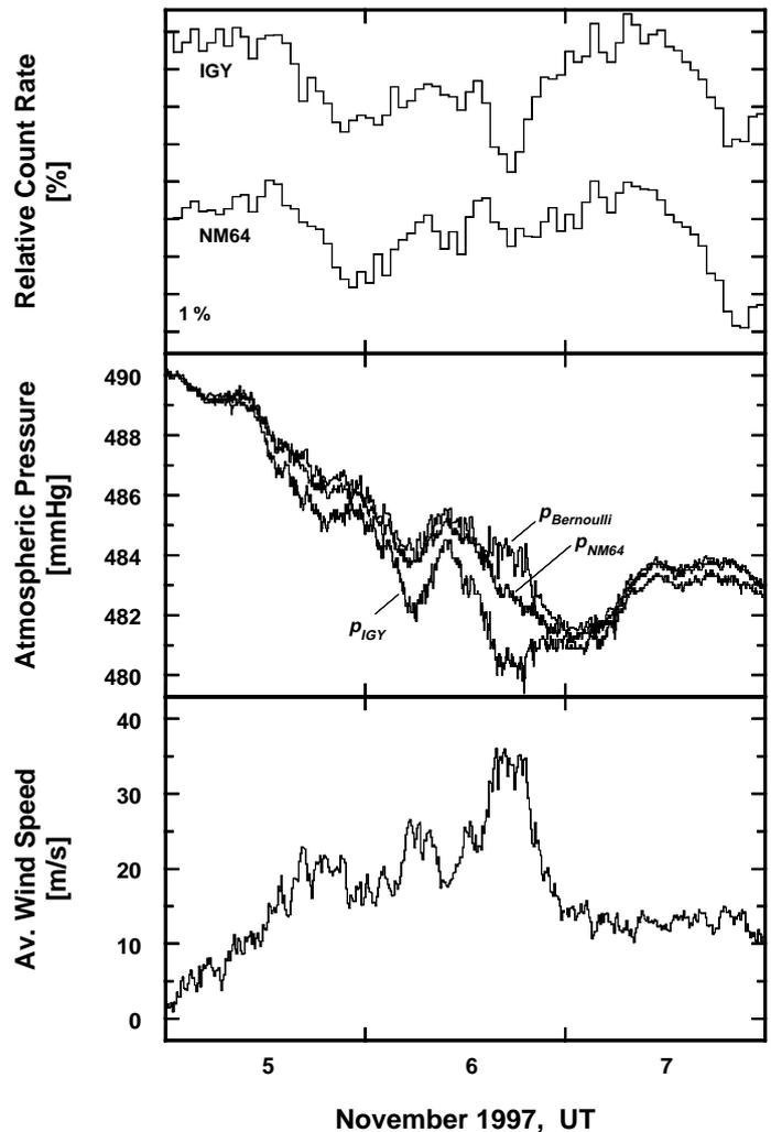
**Figure 1:** Top panel: Relative count rate of the IGY and NM64 NMs at Jungfrauoch (hourly values). Middle panel: Atmospheric pressure at Jungfrauoch. Measurements at IGY NM and at adapted NM64 location,  $p_{IGY}$ ,  $p_{NM64}$  (5-minute values). Measurements at IGY NM location corrected for Bernoulli effect,  $p_{Bernoulli}$  (10-minute values). Bottom panel: Averaged wind speed (10-minute values). For details see the text.
