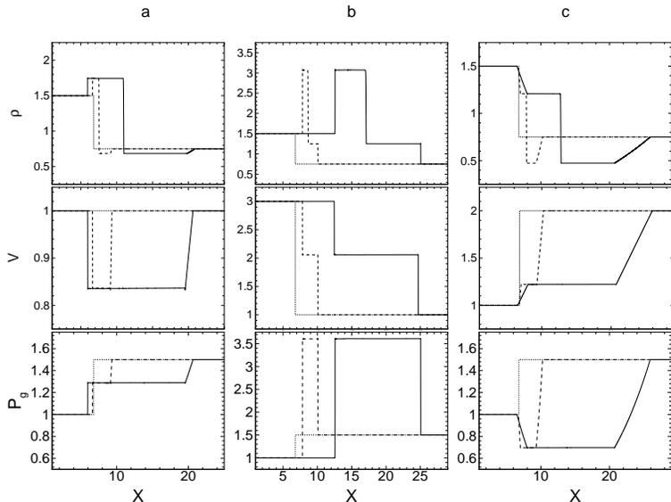
**Figure 1:** Gasdynamic Riemann problem solutions for the three cases discussed in the text. The gas density, flow velocity, and pressure are plotted.
