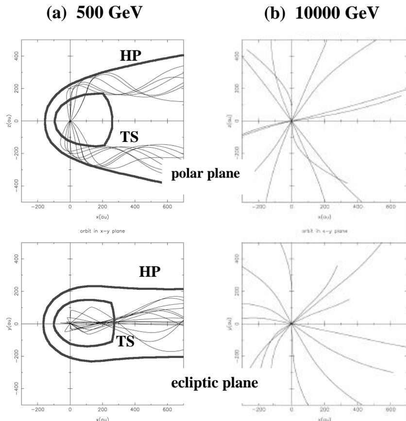
**Figure 1:** Orbits of 500 GeV (a) and 10000 GeV (b) cosmic-rays in the MHD model heliosphere. Top and bottom panels show the projections of orbits on the polar and ecliptic planes, respectively. The approximate positions of the heliopause (HP) and solar wind termination shock (TS) are indicated by thick lines in (a).
