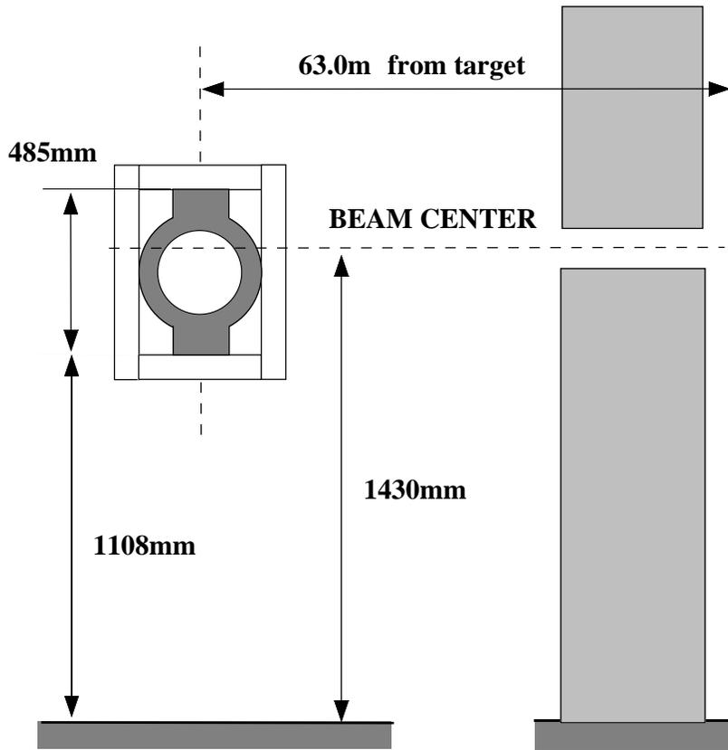
Figure 3: Arrangement of experiment (not in scale). Neutron monitor was located at 63m away from the Li target.
