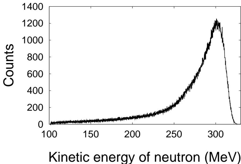
Figure 1: Energy distribution of neutrons produced by  $\text{Li}(p,n)\text{Be}$  reaction at incident protons with 300MeV.
