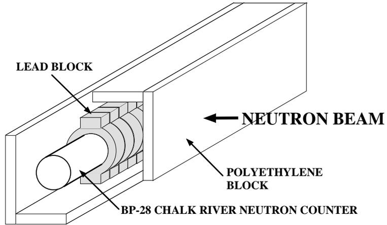
Figure 2: Schematic view of the neutron monitor which we used at the experiment.
