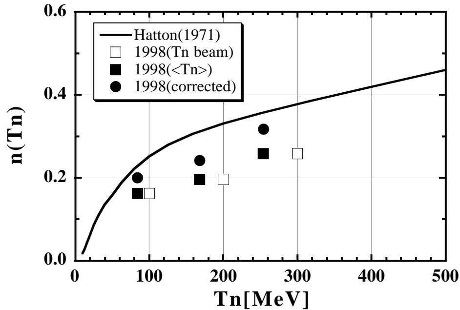
Figure 4: The detection efficiency (vertical axis) of the neutron monitor is shown as a function of the neutron energy.
