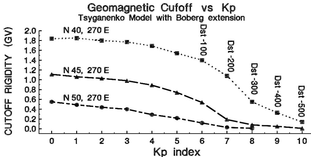
Figure 1. Illustration of the cutoff reduction at various magnetic activity levels. The coordinates are the locations of the lowest cutoff value experienced by the ISS orbit at the specified latitude in the Northern Hemisphere.
