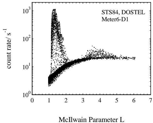
**Figure 4:** Count rate on STS81 (left) and STS84 (right) versus L-parameter in 390 km altitude.
