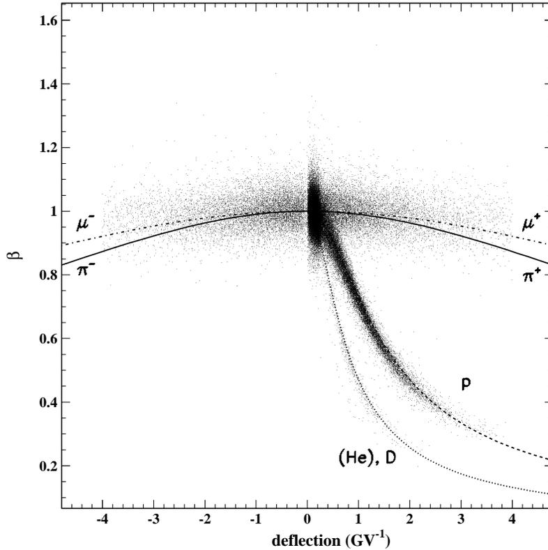
**Figure 2:** Velocity measurement from the ToF system as a function of magnetic deflection for particles collected during the ascent of the flight.
