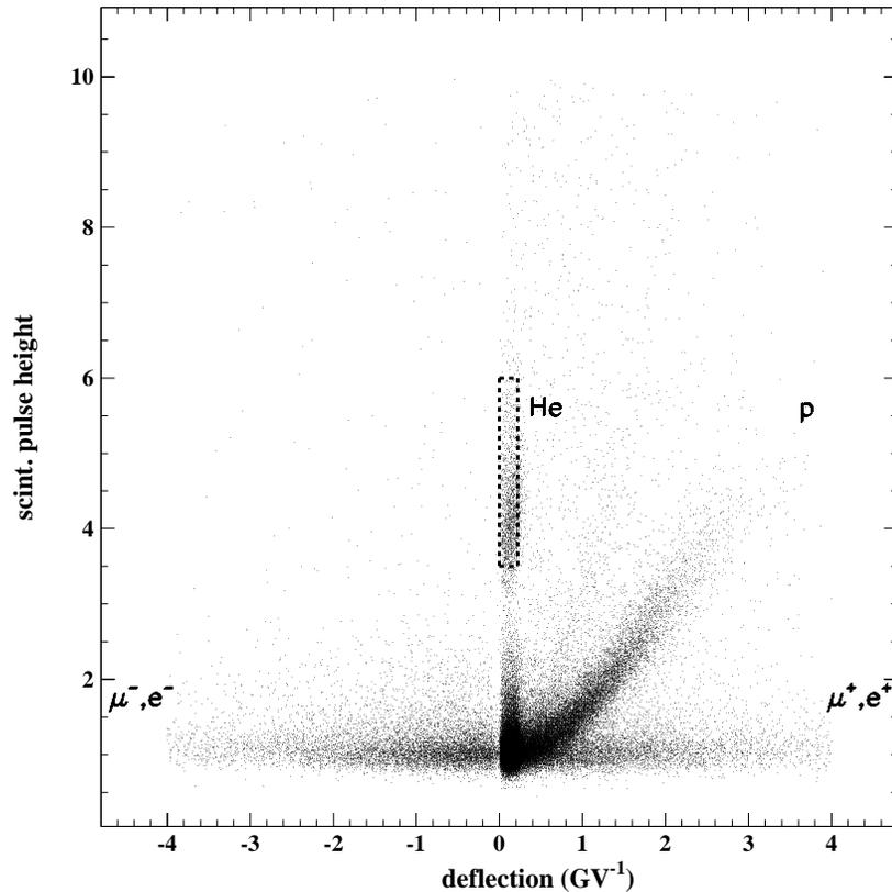
**Figure 1:** Scintillator pulse height as a function of magnetic deflection for particles collected during the ascent of the flight. The scintillator signals have been normalized with respect to the average signals from minimum ionizing singly charged particles. The helium selection is shown by a dashed line. The number of events in this plot, as well as in Fig. 2, is 56 944.
