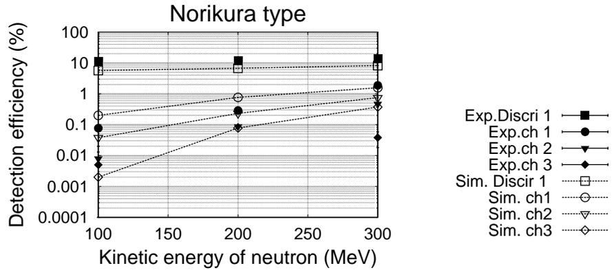
Figure 3: Detection efficiency of the Norikura type neutron telescope.
