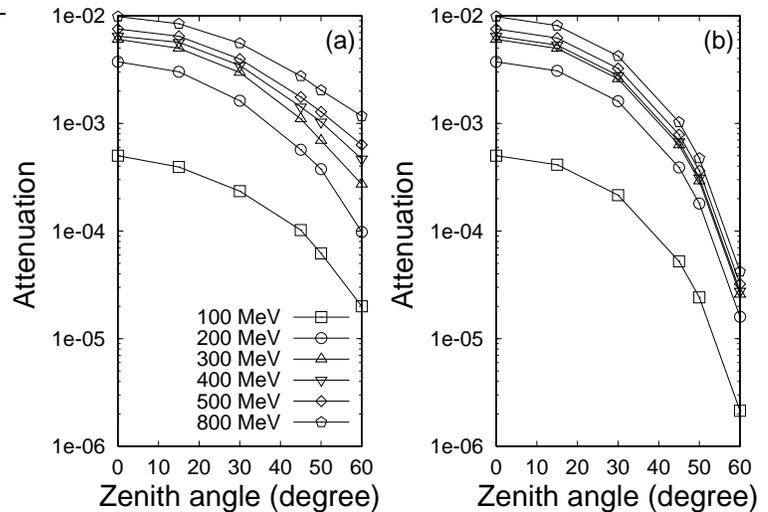
Figure 4: The result of Monte Carlo calculation for the attenuation of neutrons in the atmosphere, (a) with the minimum path length effect and (b) without the minimum path length effect at 4300m altitude.
