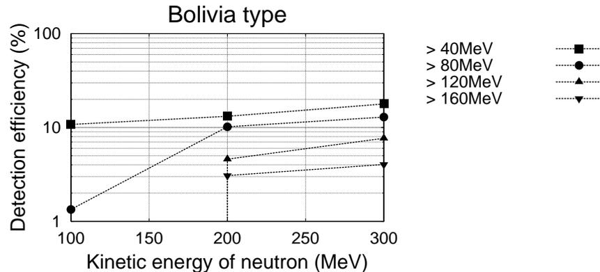
Figure 1: Detection efficiency of the Bolivia type solar neutron detector.
