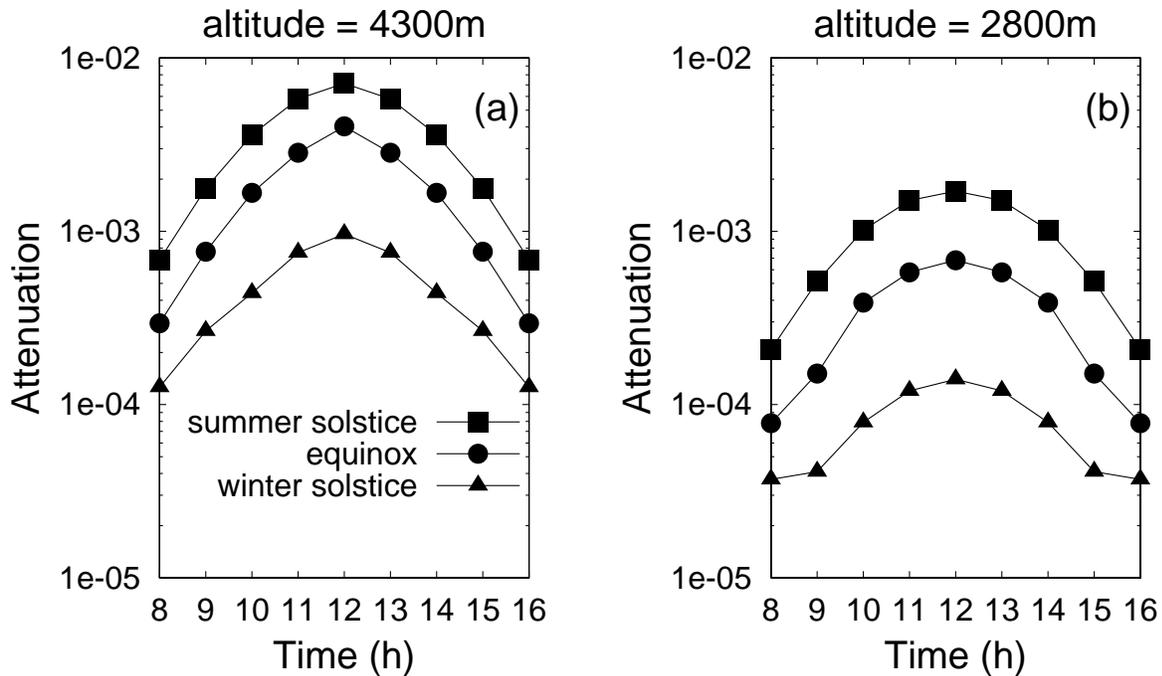
Figure 5: Daily attenuation curve for neutrons with 500MeV at two observation points.
