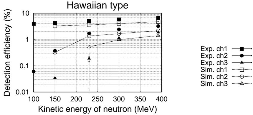
Figure 2: Detection efficiency of the Hawaiian type neutron telescope.
