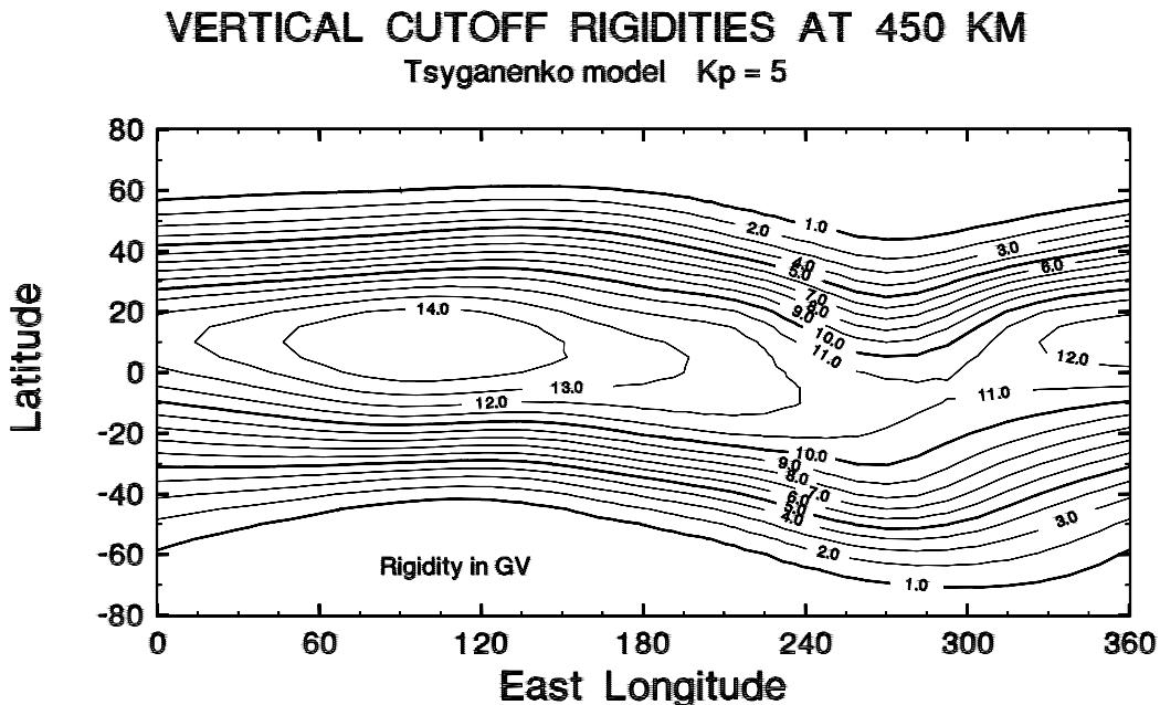
Figure 1. Cutoff rigidity contours at 450 km altitude for active ( $K_p = 5$ ) magnetic conditions.
