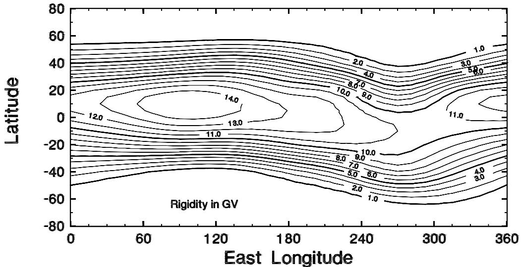
Figure 2. Cutoff rigidity contours at 450 km altitude for disturbed ( $K_p = 5$ ,  $Dst = -300$ ) magnetic conditions.
