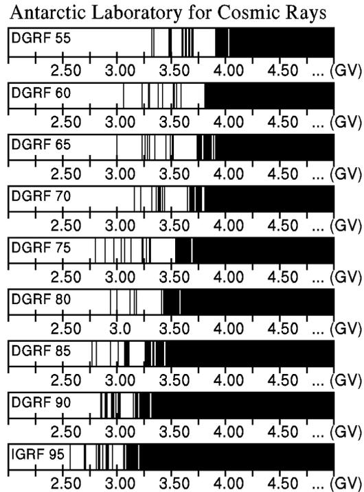
**Figure 2:** Charged particle access at LARC location. Allowed particle rigidities are reported as dark areas and the forbidden ones by white areas.
