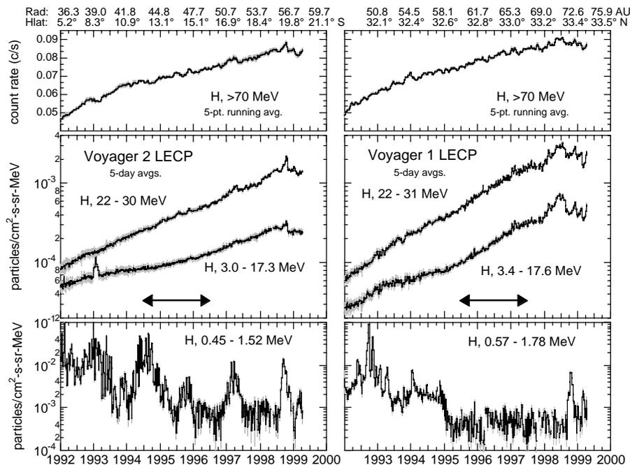
**Figure 1:** Overview of selected proton (H) channels from Voyager 2 (left) and Voyager 1 (right) during 1992-1999.3.
