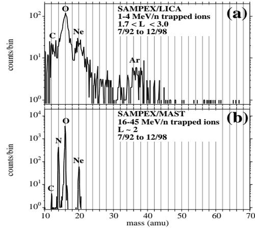
**Figure 1.** Trapped ion mass spectra at low & high energies.
