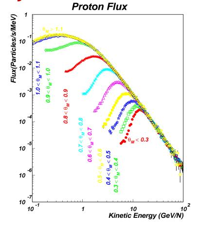
Minimum rigidity (p/Z) depends on magnetic latitude  $\Rightarrow$  cutoff in the spectrum of cosmic particles
