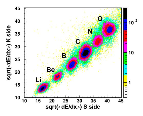
Nuclei range from lithium to oxygen in the rigidity interval 1 GV to 100 GV
