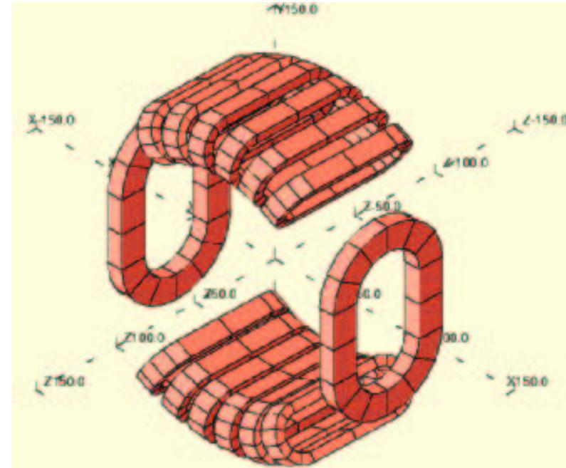
12 racetrack coils + 2 dipole coils
