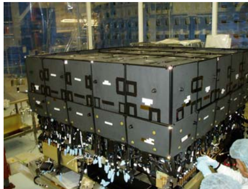
Figure 6. ACD in final phase of integration. Two bottom tile rows are not installed yet (to show fiber cables and PMTs)
