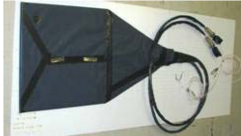
Figure 4. Scintillating tile with two fiber bundles (prototype)
