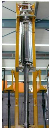
Liquid metal spallation target
