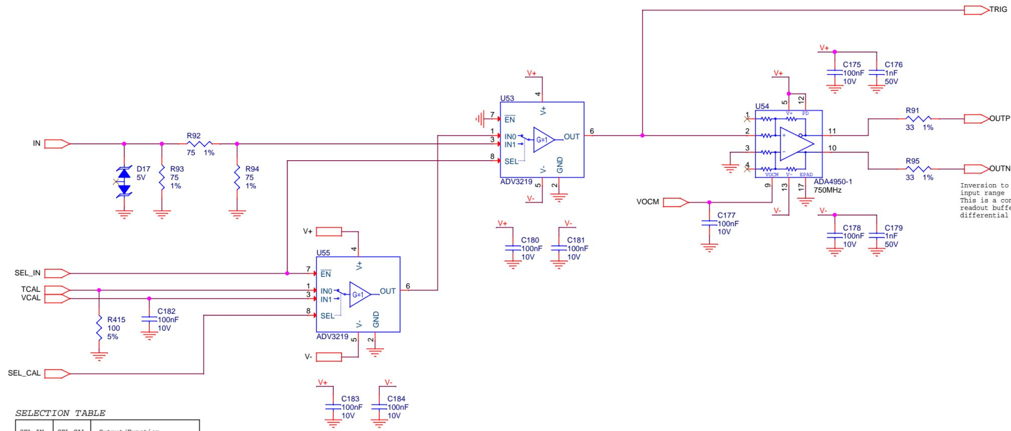
Inversion to allow a -0.9V to +0.1V input range
