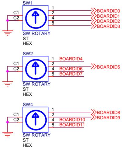
FPGA I/O NEED TO BE CONFIGURED WITH PULL-UP AND BOARDID BE INVERTED TO REFLECT CORRECT ENCODING
