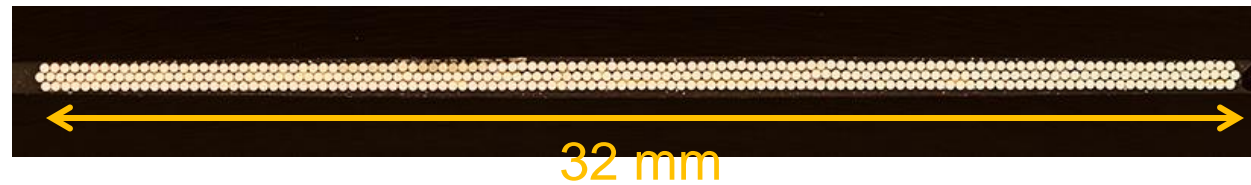
ribbon profile: 3 \times \sim 125 fibers (prototype)
