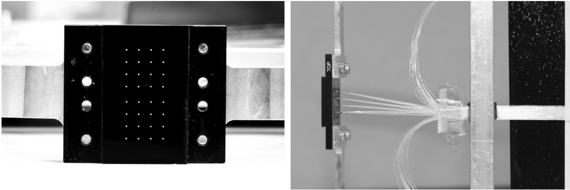
Figure 3.9 – Front (Left) and lateral (Right) view of the single fiber fanout connector.
