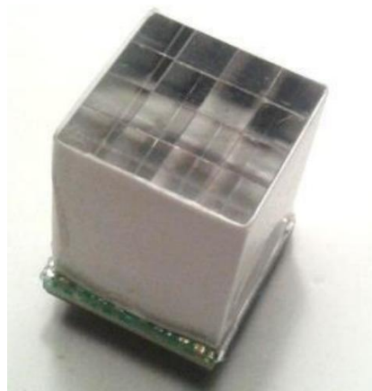
(b) Outer plate crystal matrix.
