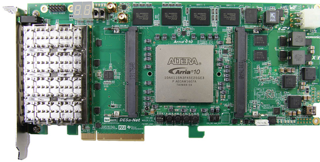
Figure 136: The DE5a NET board built by Terasic Inc. and used as a receiving board in the filter farm PCs. The Arria 10 FPGA with a PCIe Gen3 8 lane interface is complemented by a 16 duplex fast optical links and several GB of DDR4 memory.
