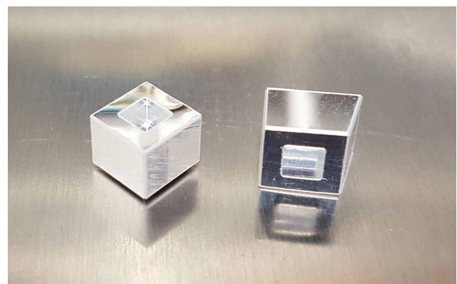
Figure 97: Individual tiles wrapped with ESR reflective foil.
