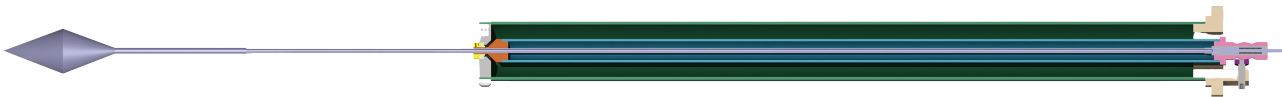
Figure 35: Cross section of target support and alignment mechanism. Muons hit the target from the left. The stopping target is mounted on a thin carbon tube which is steered and fixed in the support structure. The rear end of the support structure consists of an alignment mechanism to adjust the position of the target.
