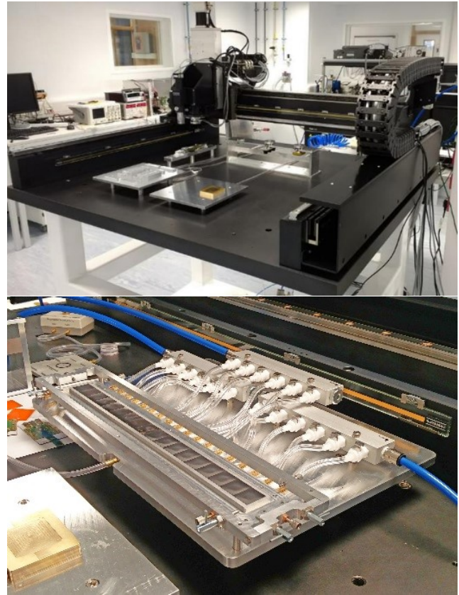
Figure 55: Robotic gantry (upper figure) for placement of 17 or 18 MUPiX chips on the vacuum jig (lower figure).
