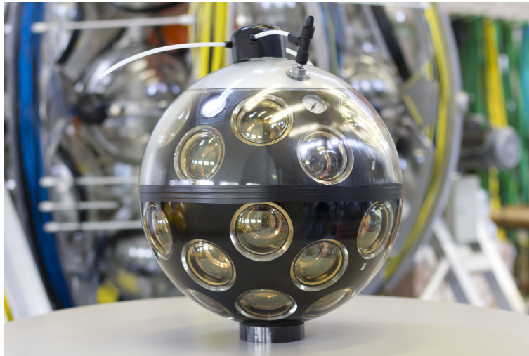
Figure 22: Prototype of a multi-photomultiplier optical module for KM3NeT. The module incorporates 31 3-inch photomultipliers, their high-voltage bases, and the electronic modules for signal digitization and communication to shore. Photograph by KM3NeT Collaboration.
