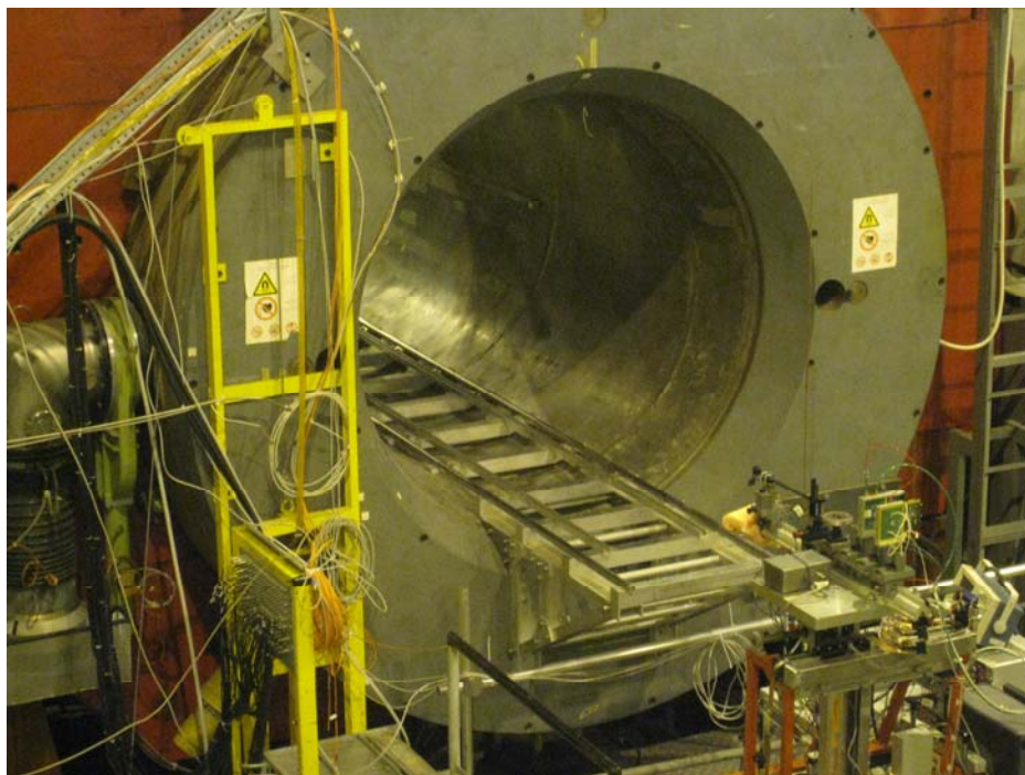
Morpurgo magnet on the H8 beam line at CERN
