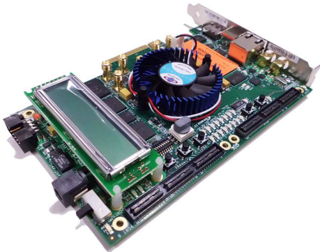
Figure 14.3: ALTERA Stratix IV PCIe development board.
