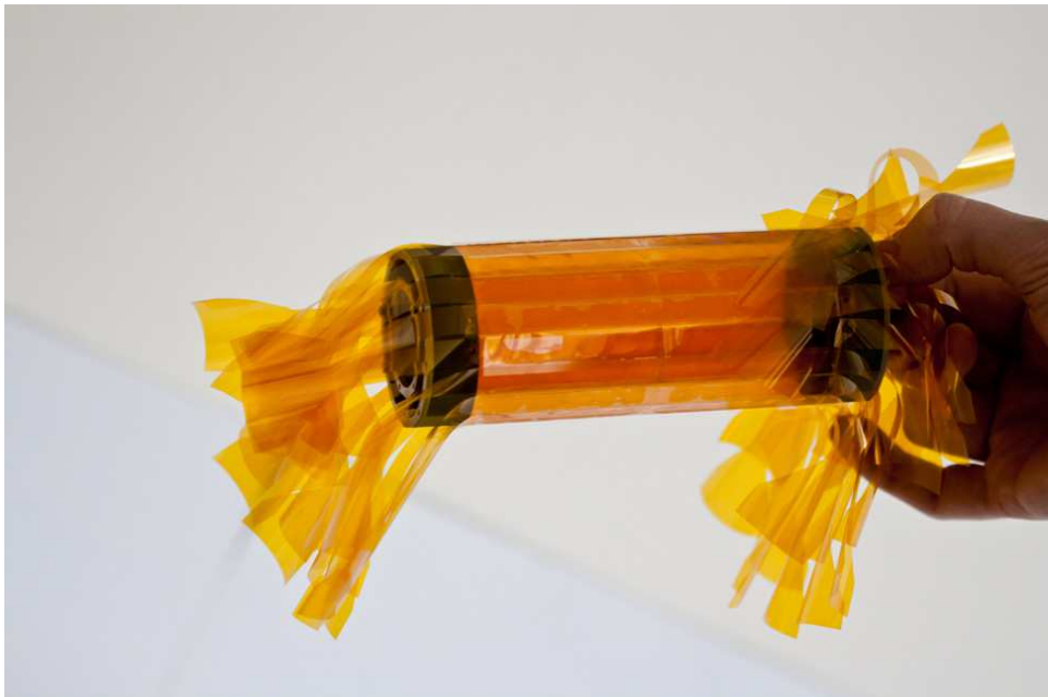
Figure 10.20: Mechanical prototype of the inner pixel layers. Thin glass plates replace the silicon chips.
