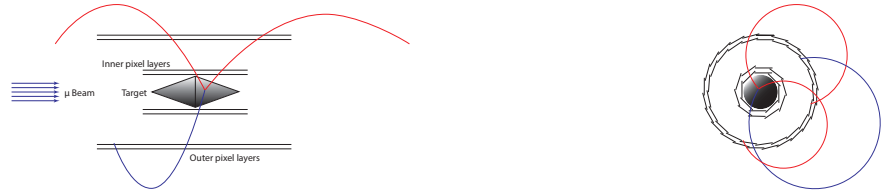
Figure 3.7: Minimum detector configuration for early commissioning with central silicon only (phase IA).
