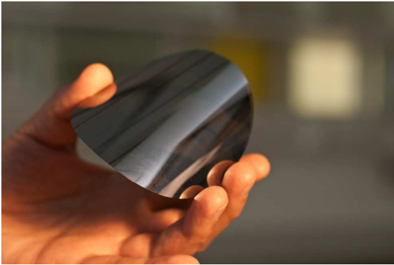
Figure 8.5: A 50 \mu\text{m} thin silicon wafer.
