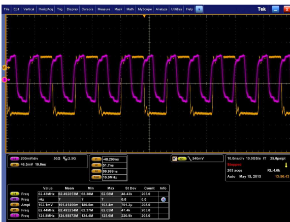
Figure 10.3: MuPix phase locked to reference clock. Orange: 62.5 MHz MuPix clock output \text{clk8n} , Purple: 125 MHz reference clock from FPGA.
