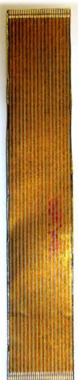
Figure 8.20: Aluminum-Kapton flex-print prototype produced in-house. The flex-print is 10 cm long and 1.8 cm wide. It comprises 17 differential signal pairs.
