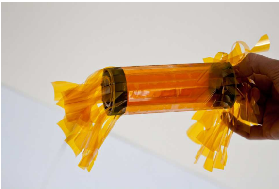
Figure 8.6: Mechanical prototype of the inner pixel layers. Thin glass plates replace the silicon chips.
