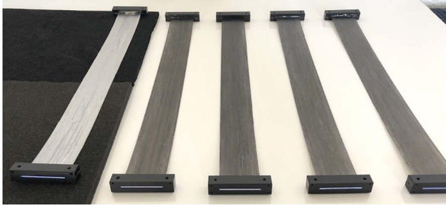
Figure 3.5: Various full size SciFi ribbon prototypes formed by staggering 250 \mu\text{m} diameter round scintillating fibers. The fibers are assembled with different adhesives (the black epoxy gives the black color to the ribbons).
